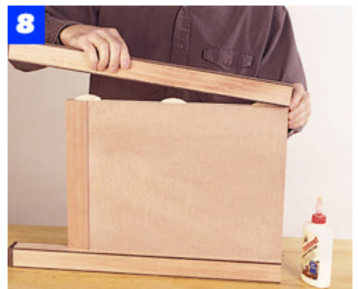
After gluing the bottom rails to the sides, use plates to join the sides and rails to the table legs.
