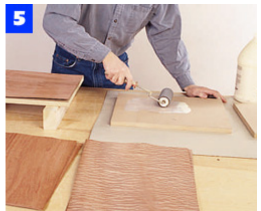
Use a foam roller to spread glue onto the cores. Aim for an even coating and do not leave pools of glue.
