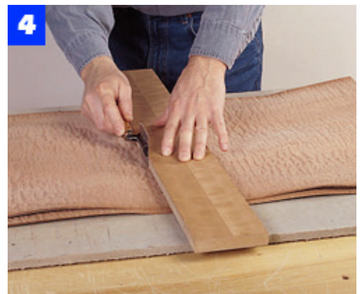
Use a straightedge to guide the veneer saw. Make light passes to avoid splitting or tearing the delicate veneer.
