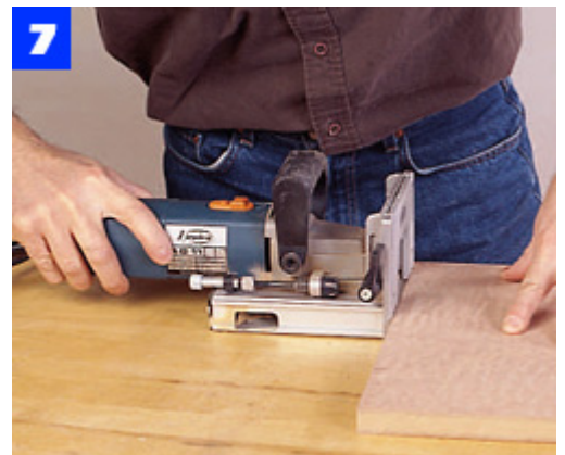
Cut plate slots in the side panels and bottom side rails. Hold the joiner and work against a table to register the cuts.
