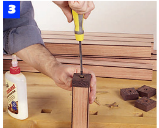
Glue and screw 3/4-in.-thick wenge foot blocks to the legs. Then, use a table saw or plane to chamfer each foot.
