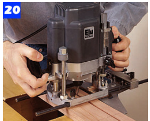
Use a 1/4-in. straight bit to rout slots for the drawer bottom. The slot in the face runs only between the dovetail slots.
