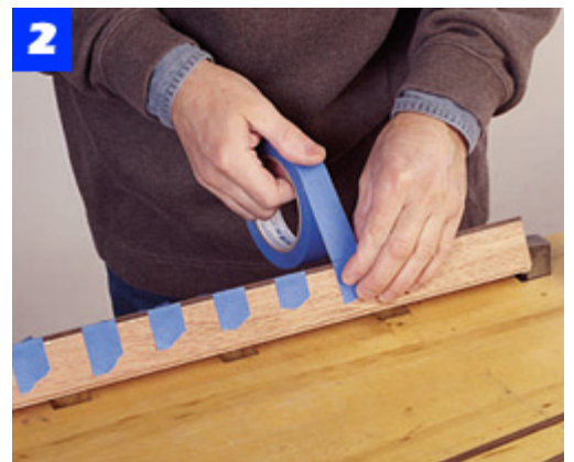
Glue the inlay strips into the leg-corner rabbets. Place masking tape every 2 in. to clamp the strip to the leg.
