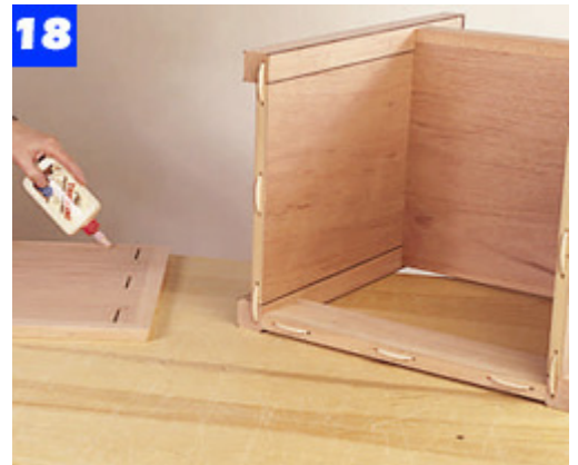
Spread glue in the slots and on joining plates for joining the top to the sides and back rail. Clamp the assembly.
