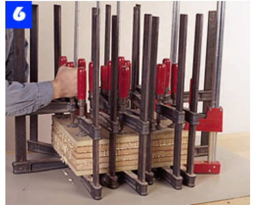
Arrange the panels in a stack with a layer of kraft or wax paper between each. Use as many clamps as possible.
