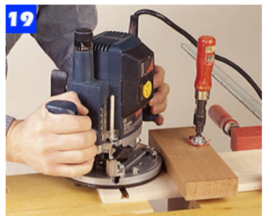
Use a 1/2-in. dovetail bit to rout the slots in the drawer face and sides. Guide the cuts with a board clamped to the work.
